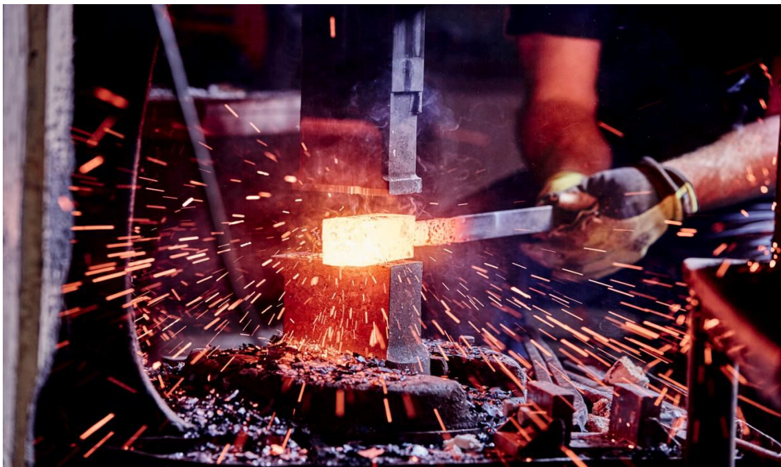
Stretching Mosaic Damascus steel on air hammer
